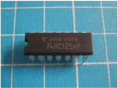
A black integrated circuit (IC) with 14 pins, labeled "JAPAN 1307H 74HC125AP". | 2 個 |
