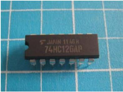
A black integrated circuit (IC) with 14 pins, labeled "JAPAN 1146H 74HC126AP". | 2 個 |
