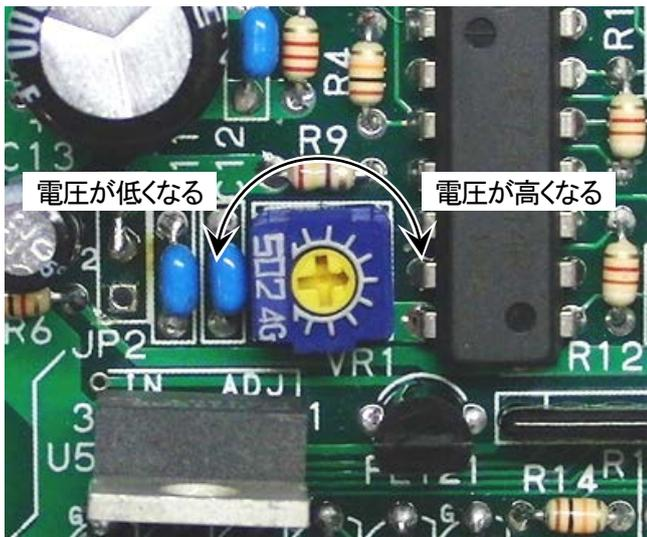
A close-up of a green PCB. A blue potentiometer labeled "512 4G" and "VR1" is mounted. Two arrows point to the potentiometer: one from the left labeled "電圧が低くなる" (Voltage decreases) and one from the right labeled "電圧が高くなる" (Voltage increases). Other components like resistors (R9, R12, R14) and a connector (JP2) are visible. | <p>VR1 で調整します。時計回りで電圧が高く、反時計回りで電圧が低くなります。</p> |
